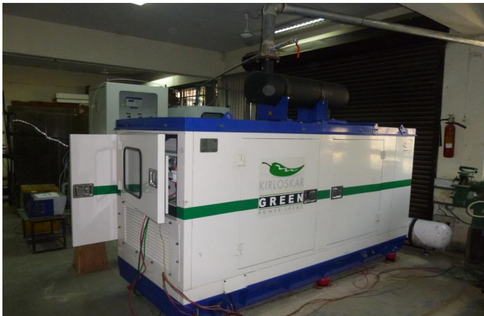
Figure 14: A photographic view of a hydrogen-fuelled generator developed in IIT Delhi with MNRE fund support.
