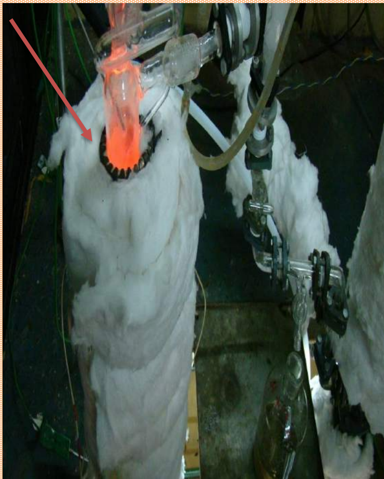
Sulfuric acid decomposer operating at 900 ° C.
