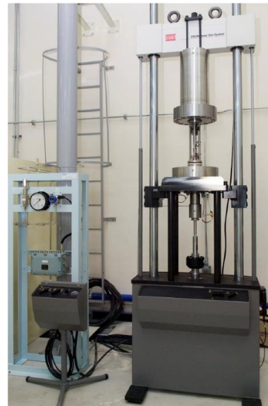
SSRT cum Fatigue testing with online H 2 Charging
