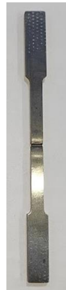
X70 Charged sample failed at notch region
