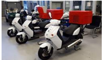
Fuel Cell powered scooters deployed at SAPO Head Office, Cape Town
